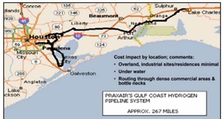
Figure 4: Linde (Formerly Praxair) H 2 Pipelines (Ehlig-Economides and Hatzignatiou 2021)
